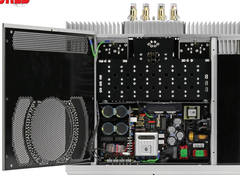
The top view shows the switch-mode power supply, with its many transformers and capacitors, is situated at front. Although switch-modes have transformers, they are not big and weighty like traditional types, because the conversion process works at high frequency.
